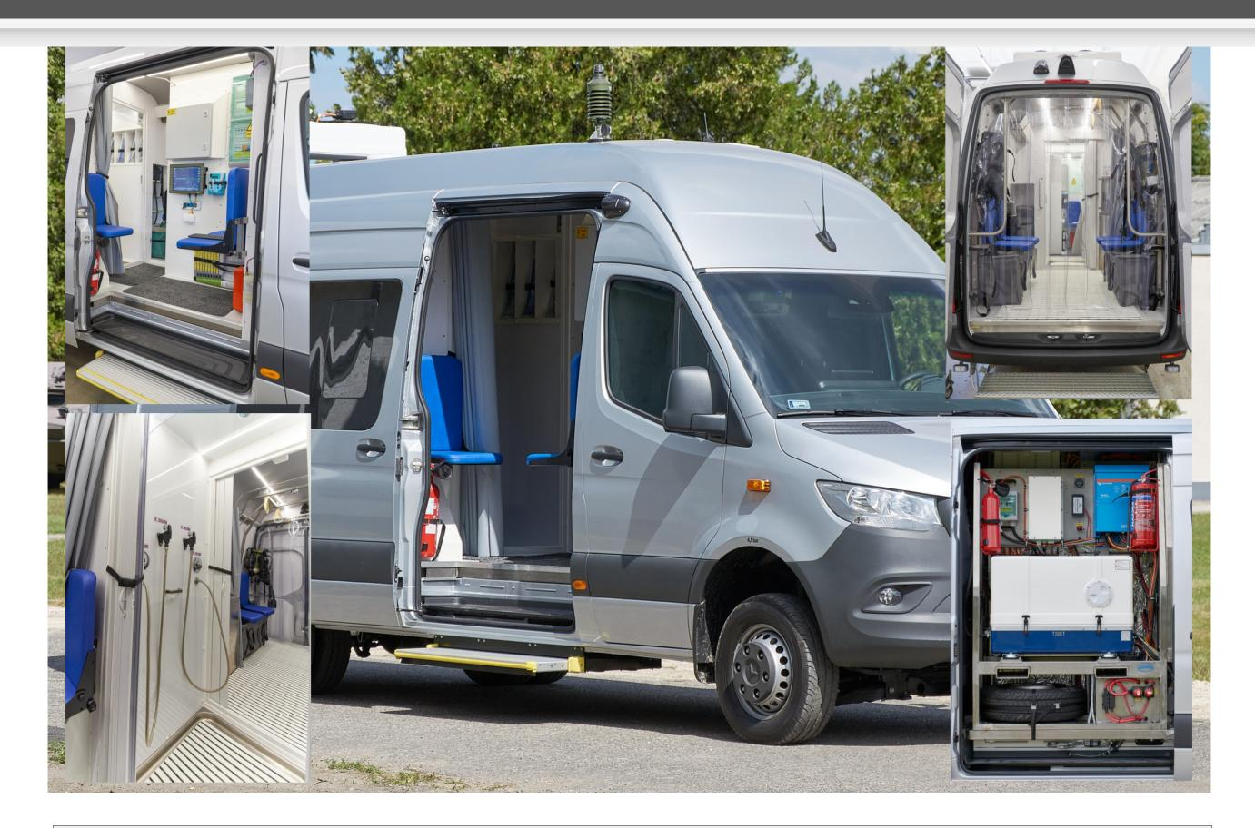
The purpose of the CBRN-E Decontamination Vehicle is the on-site decontamination of intervening personnel and their equipment after the execution of CBRN-E related tasks.
