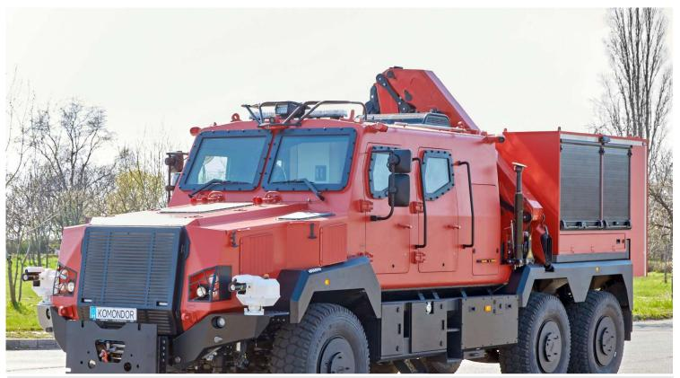
GMMF-20 Technical recovery superstructure: 11 t meter hydraulic crane Lift-tow fork with up to 8 t capacity 5 kVA electric power generatorHydraulic power rescue set38 t towing ability
