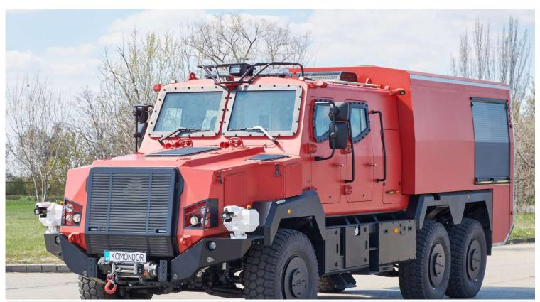
VCSF 7000 Firefighter superstructure: 7000 I water tank with fire-fighter pump Remote controlled front nozzles
